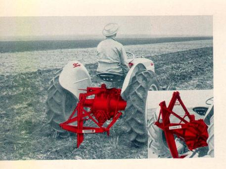
Many times when you ordinarily use a plow, this Dearborn Subsoiler will do a better job. For instance, plows are sometimes used to loosen gravel or hard-packed sand prior to loading. By using the Subsoiler, you do a deeper and better job-also save points and moldboard wear.
