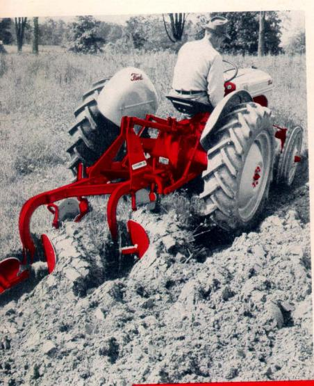
Note that the Dearborn Plow is carried by the Ford Tractor. In effect the rear wheels of the tractor become wheels for the plow. No need for wheels or axle on this plow either in transport or in the field. In the Dearborn Plow they would be worse than useless!
