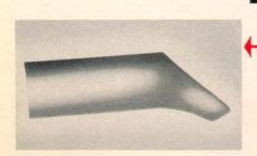
Full cut or regular shares are adaptable to average soil conditions and are most widely used. They assure a clean cut furrow slice.
